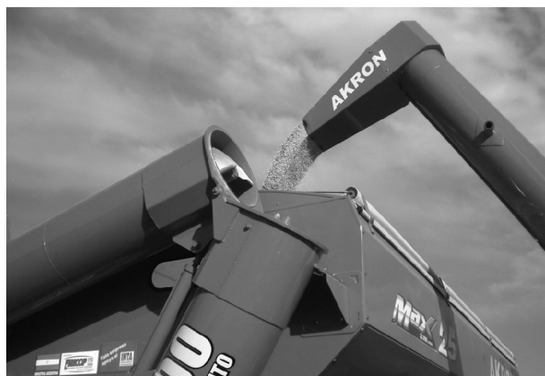
Figure 6.2 Grain discharge into the grain cart.
